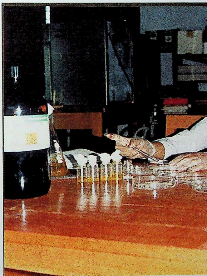
Fig. 8. Application of doses for insecticidal test.
