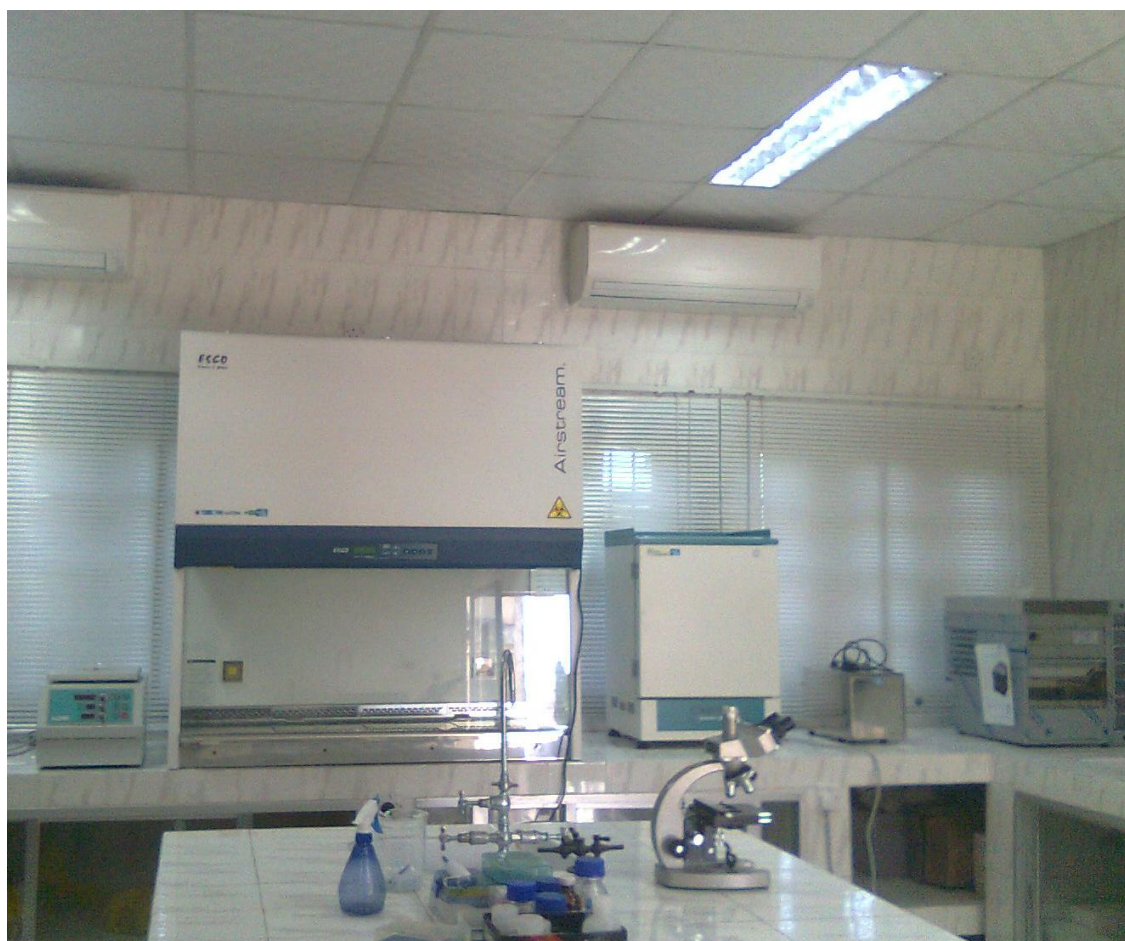
Plate 2.7: Biological safety cabinet in BCSIR microbiology laboratory, Rajshahi
