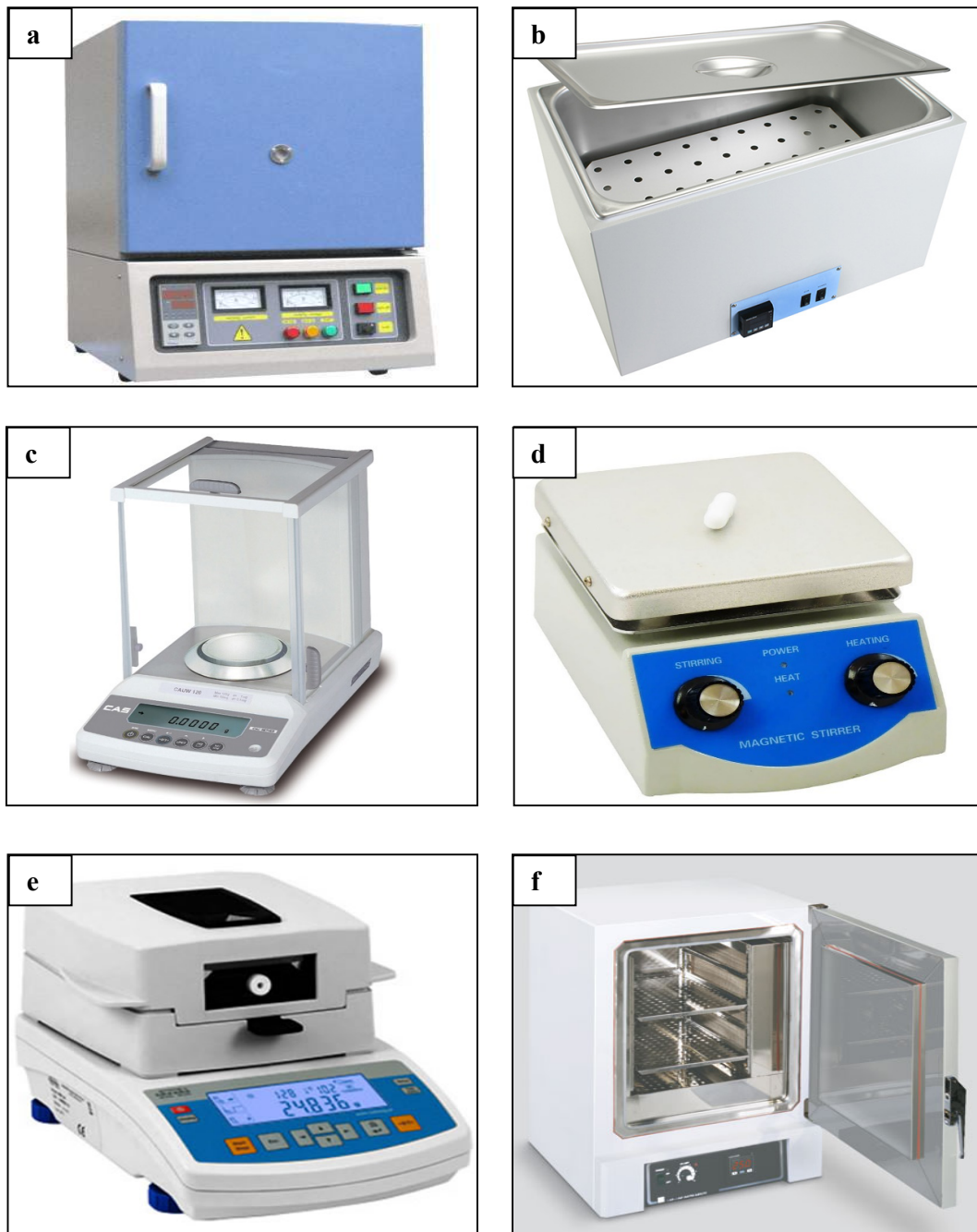
Figure 2.2: Instruments used in the present investigation (a) Muffle furnace, (b) Water bath, (c) Electronic balance, (d) Magnetic stirrer, (e) Moisture analyzer and (f) Forced convection oven.
