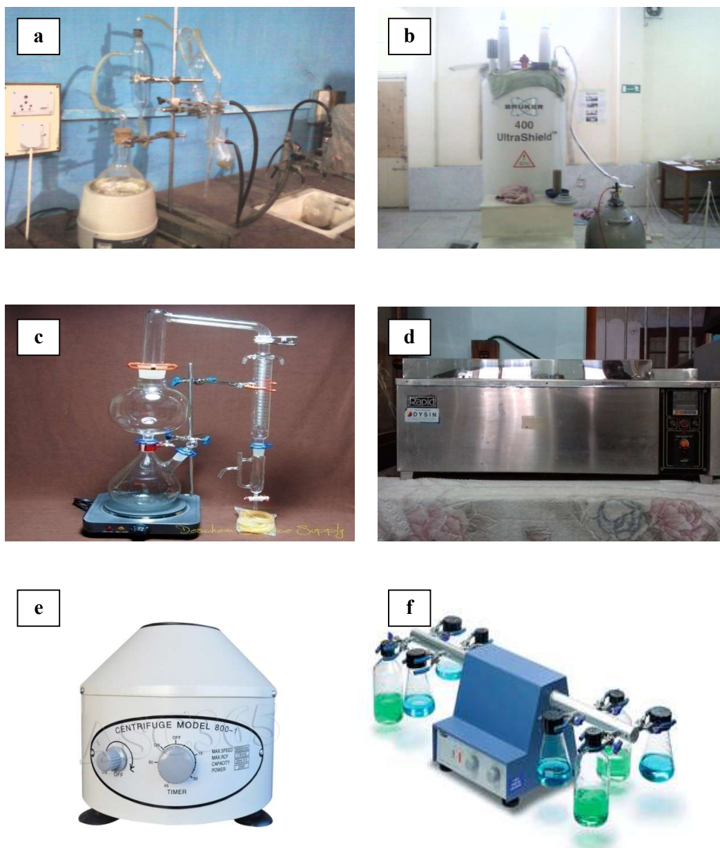
Figure 2.1: Instruments used in the present investigation (a) Kjeldahl machine, (b) NMR spectrometer, (c) Reflux system, (d) Dye bath, (e) Centrifuge machine and (f) Shaker
