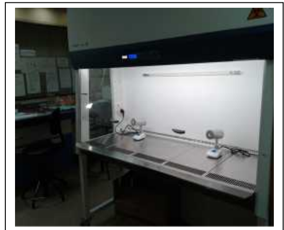
Fig.-8.6: Biosafety Cabinet for microbial culture
