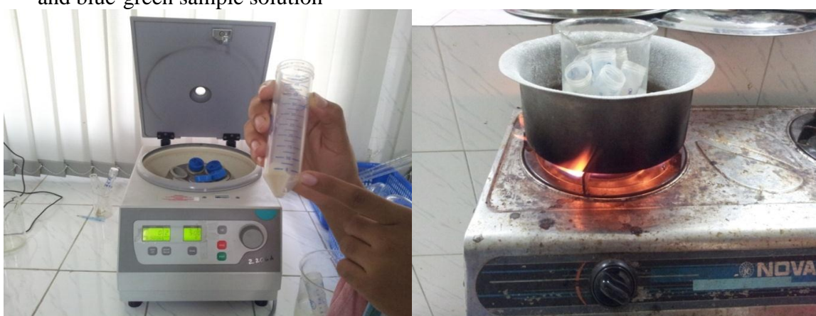
C: Precipitate collected by centrifugation
