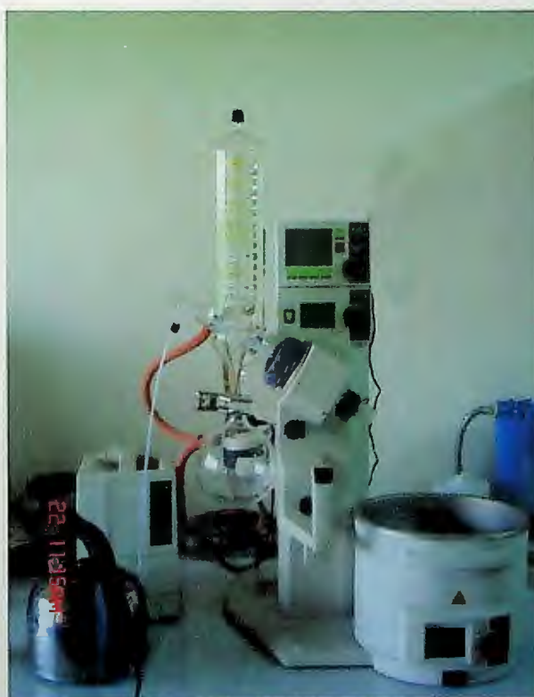
Plate 15 : Evaporation of mixed solvent from extraction by a Vacuum Rotary Evaporator ( Rota vapor R-215 )
