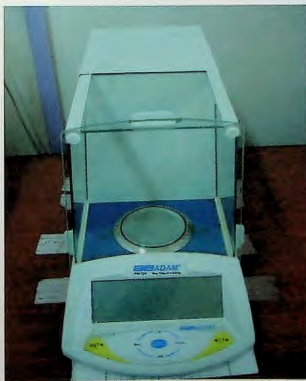
Plate 7 : An Electronic Balance (ADAM R PW-124)
