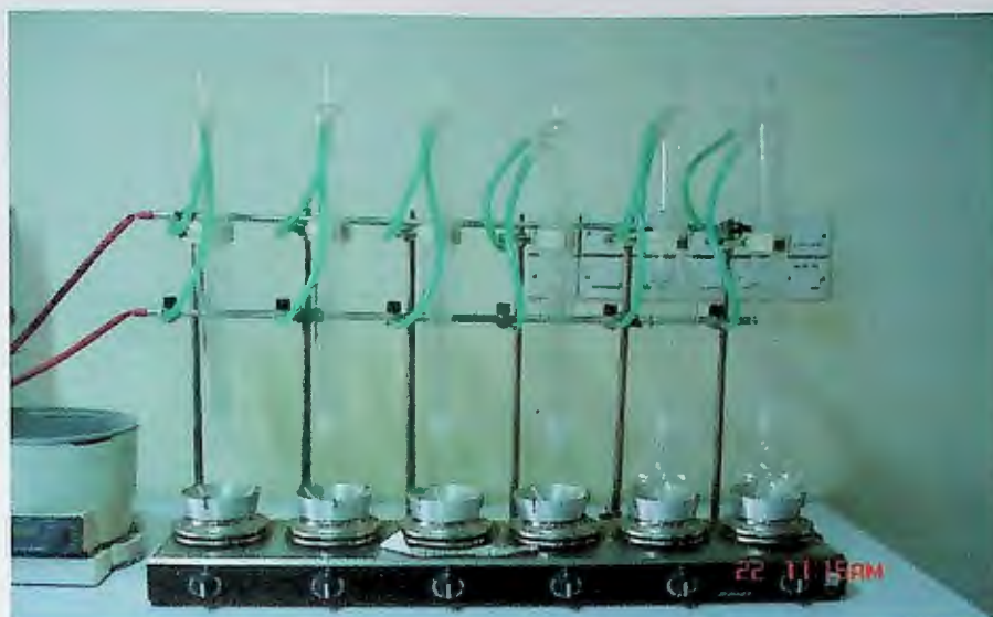
Plate 14 : Plant parts extraction in a Soxhlet's apparatus ( Type: EV-16 )
