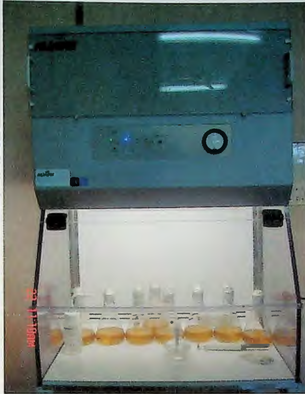
Plate 16 : Laminar Air Flow Unit (Model No. NU- 126-300E)
