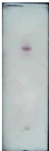
Figure 2.1 Purity of compound-1 on TLC plate using the solvent system of n-hexane and ethyl acetate (9 : 1)
