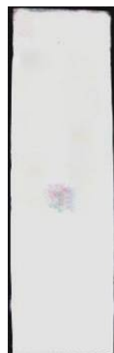
Figure 2.5 Purity of compound-5 on TLC plate using the solvent system of n-hexane and ethyl acetate (19 : 1)
