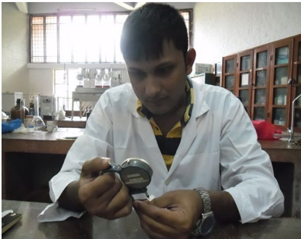
C Measuring shell thickness
