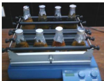
Fig 12. Shaking for extraction
